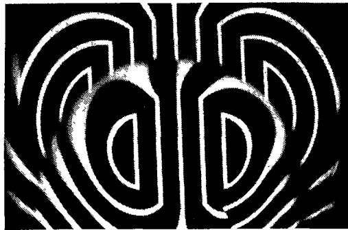
Fig.6 inside surface reflection of two cylinder mirrors
