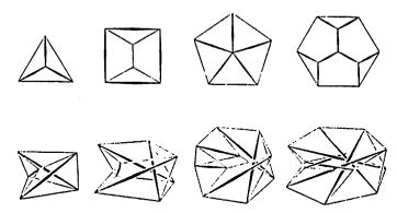
The stable simplex is an autonomous equilibrium which maintains itself as an indeformable entity in a non-monolithic system, thus composed essentially of compression or tension bars, assembled by movable joints.
